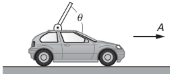
Figure 1: Pivoted rod on an accelerating car. The rod makes an angle \theta with the horizontal.
